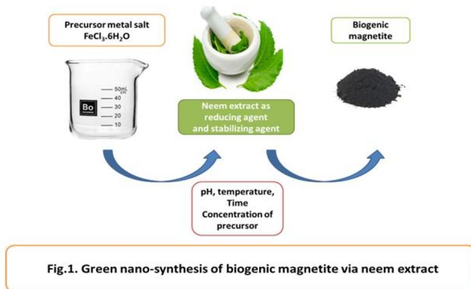
Fig.1. Green nano-synthesis of biogenic magnetite via neem extract
